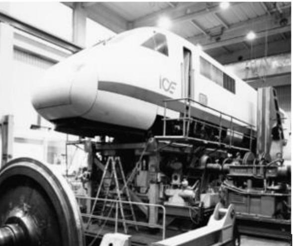
The roller rig built by DB-AG in Munich [1], [4]
